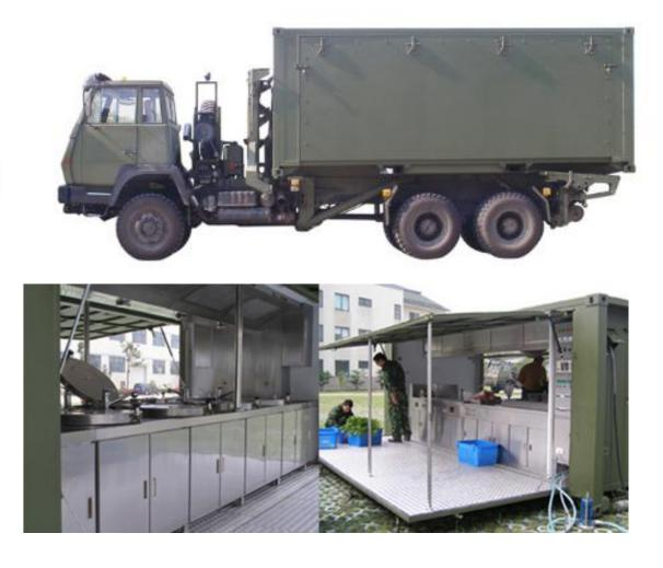
FKC-1200 Mobile Field Kitchen Container , this container can be loaded onto the truck and transported by truck platforms.
